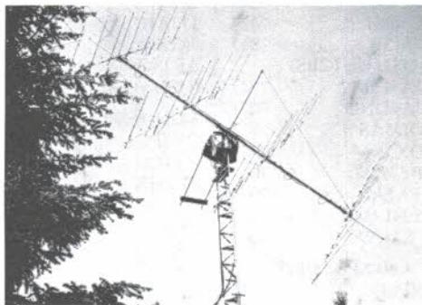
VE7BQH rotated 40° in polarity
