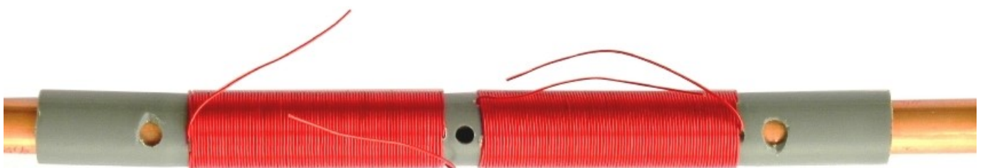
Copper tubes inserted into the PVC center-section
