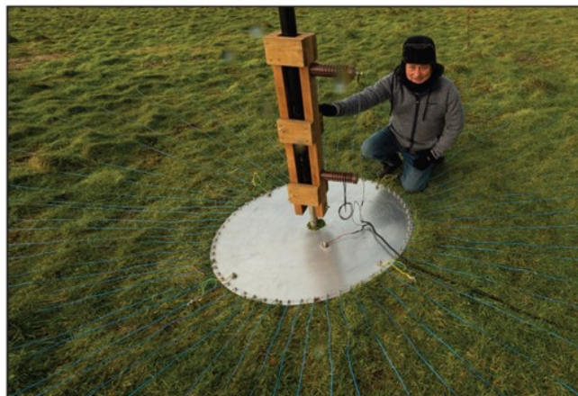
The MJ5E Topband vertical antenna radial plate with 2400 meters of radials.
